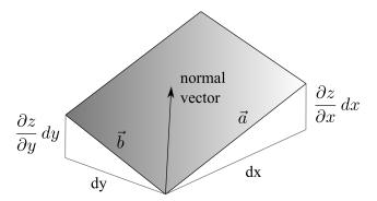
The vectors  $\vec{a}$  and  $\vec{b}$  which are the sides of the parallelogram are tangent to the surface at the point of tangency. Consider  $\vec{a}$ . It runs in the x-direction. A small change dx in x produces a change in z — the amount the vector  $\vec{a}$  "rises".
