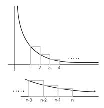
Divide the interval [1, n] up into n equal pieces, and build a rectangle on each piece, using the left-hand endpoints of each subinterval to get the heights. As you can see from the picture, the rectangles all lie above the curve, so the sum of the rectangle areas will be greater than the area under the curve.
