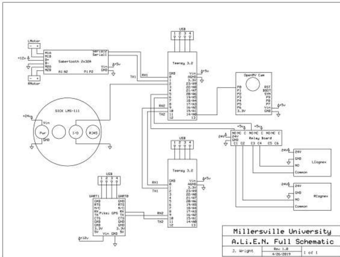
Figure 4: Full electronic schematic.
