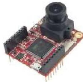
Figure 9: OpenMV Cam M7.<sup>6</sup>
