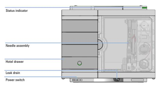
Figure 4 Overview of the Multisampler
