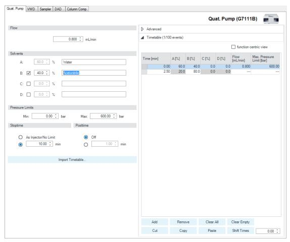
Figure 26 Timetable settings 1260 Infinity II Quaternary Pump (G7111B)
