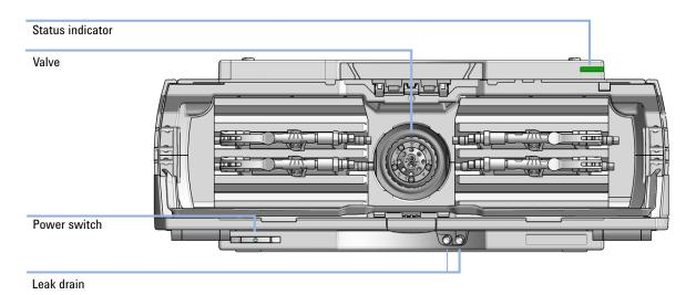
Figure 6 Overview of the Multicolumn Thermostat
