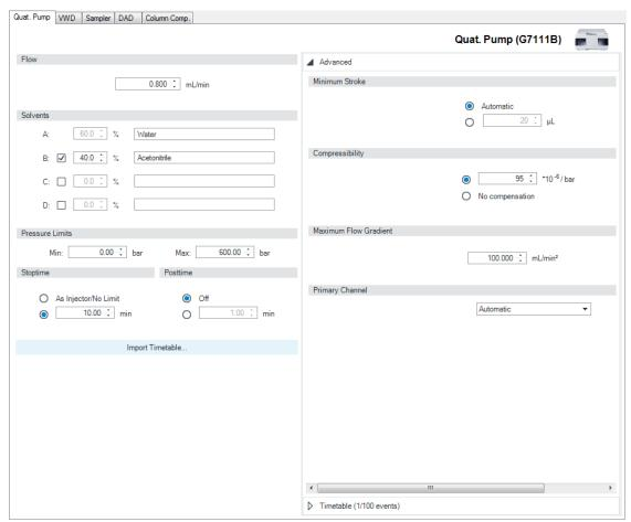
Figure 25 Method settings 1260 Infinity II Quaternary Pump (G7111B)
